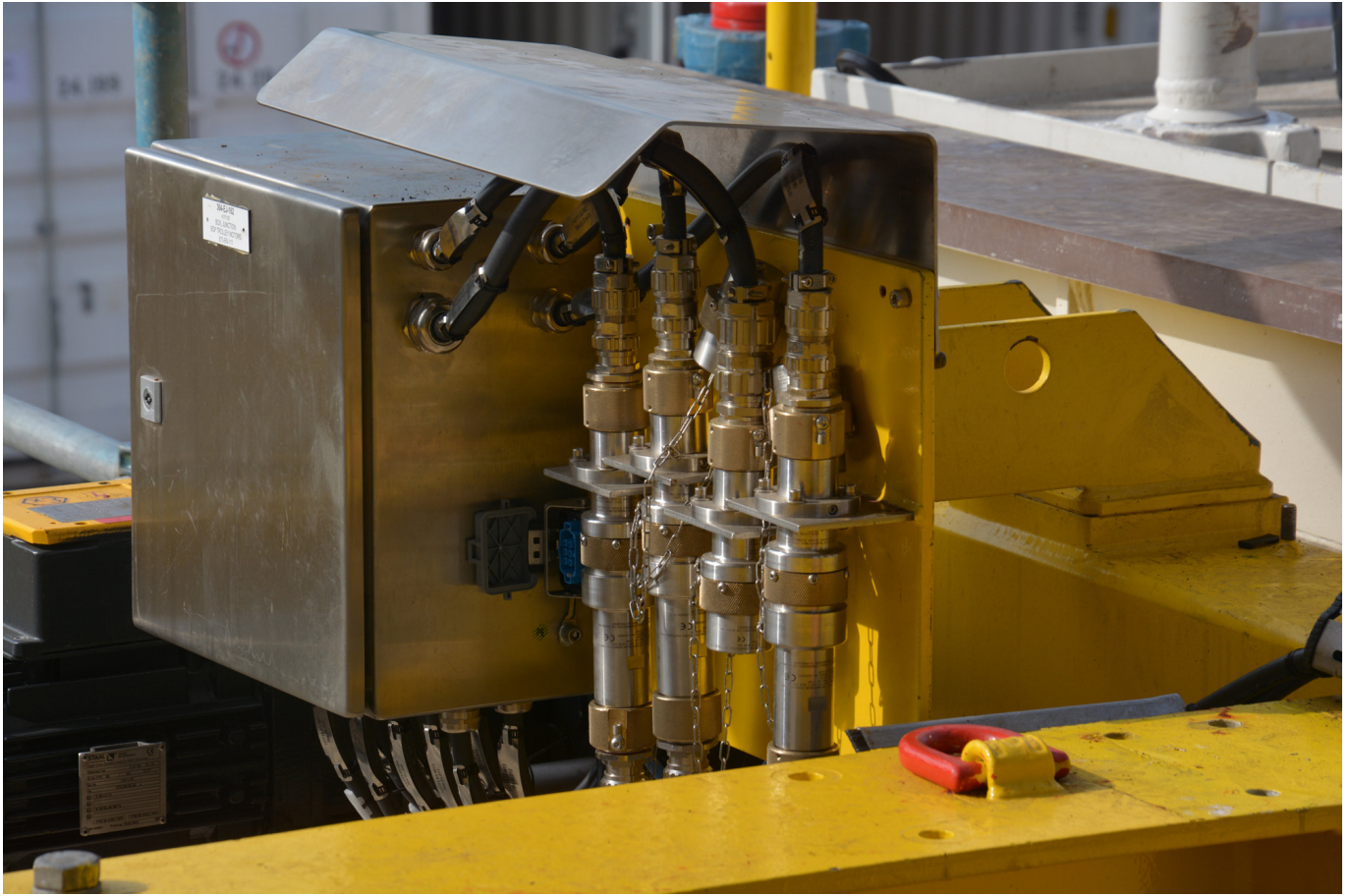
Fig. 2: HAWKE connectors make the modular concept of the VDD 400.2 offshore deep drilling rig a reality. (Photo: Jacob)
