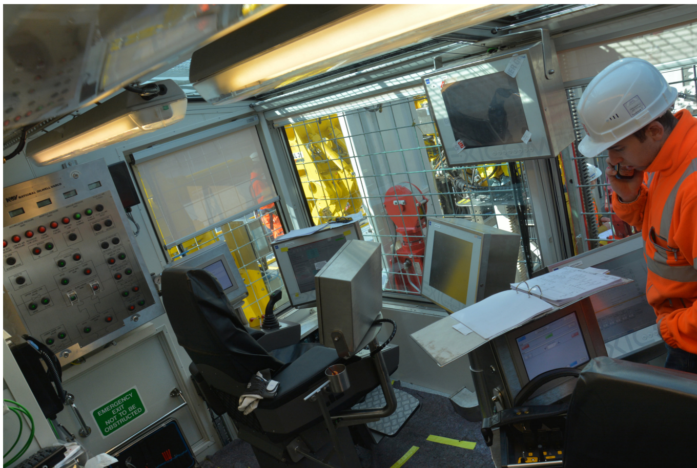
Fig. 6: The control centre of the VDD 400.2 offshore deep drilling rig (photo: Jacob)
